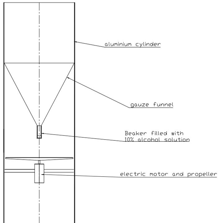
**Figure 2, Schematic Sketch of the Suction Trap used on D-4**
